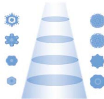
At greater depths, a conventional 7-crystal transducer has a narrower focal region.
